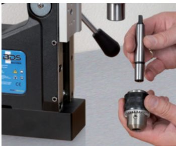
1. Connect taper drift to drill chuck.
