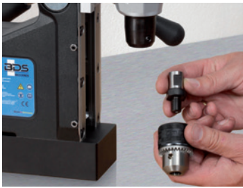
1. Connect adapter to drill chuck.
