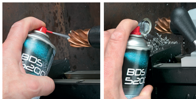
Step 1: Prior to drilling, spray high-performance lubrication spray directly into the drill.
